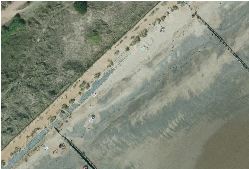
Figure 7: Erosion to the seaward side of the paling fence protecting the dunes behind, between groyne 3-4.
